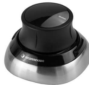
(b) SpaceMouse® 6-axis joystick
