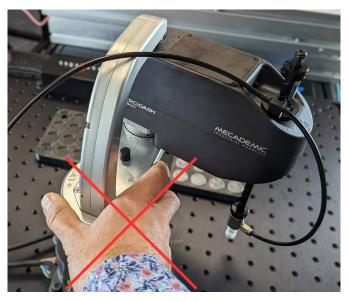
Figure 3: Pinch point between distal and proximal links
