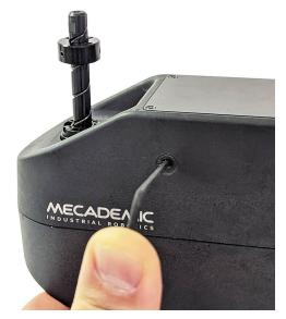
(a) Remove the screw cap
