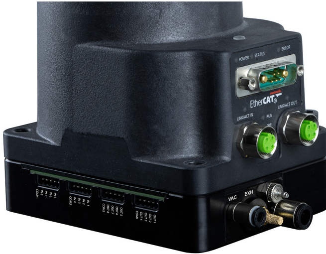
(a) MCS500 (R1) inserted onto the MVK01
