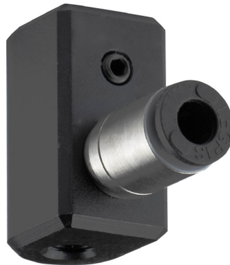
Figure 3: Suction cup holder to be attached to the flange of the MCS500, with M3 set screw, push-in pneumatic fitting for 4-mm (OD) tubing and an M5-threaded hole for installing a suction cup
