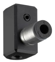
Figure 3: Suction cup holder to be attached to the flange of the MCS500, with M3 set screw, push-in pneumatic fitting for 4-mm (OD) tubing and an M5-threaded hole for installing a suction cup
