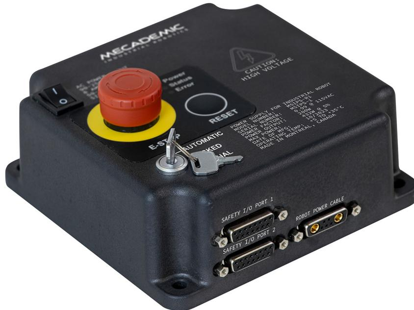
Figure 22: The MCS500 smart power supply unit (PSU), MSIPS
