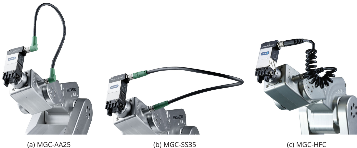
Figure 7: MEGP 25E gripper installed with the three different cables (fingers not shown)
