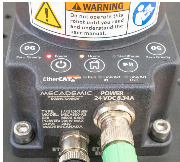
Figure 19: Robot control panel
