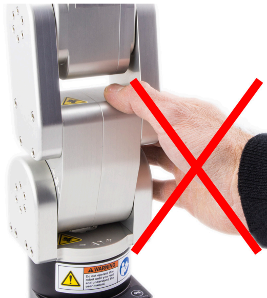
Figure 2: Keep your fingers away from the three pinch points of the Meca500
