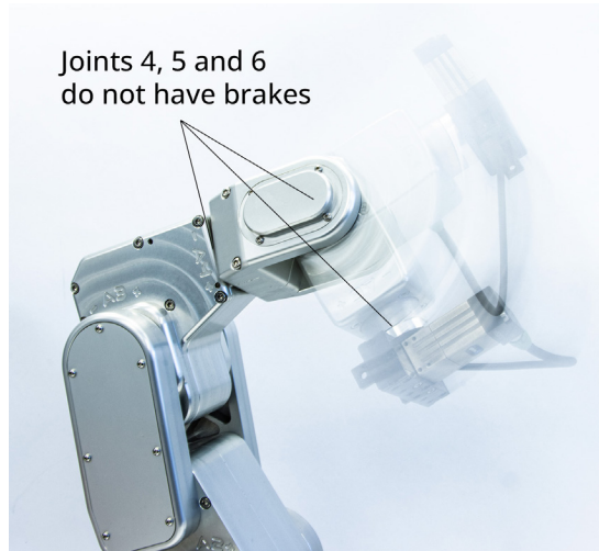
Figure 7: When the robot is deactivated, the end-effector will slowly move downwards under the effects of gravity
