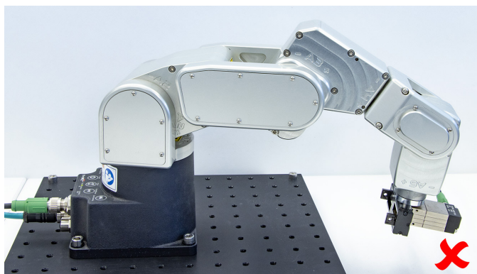
(a) DO NOT leave the robot deactivated like this
