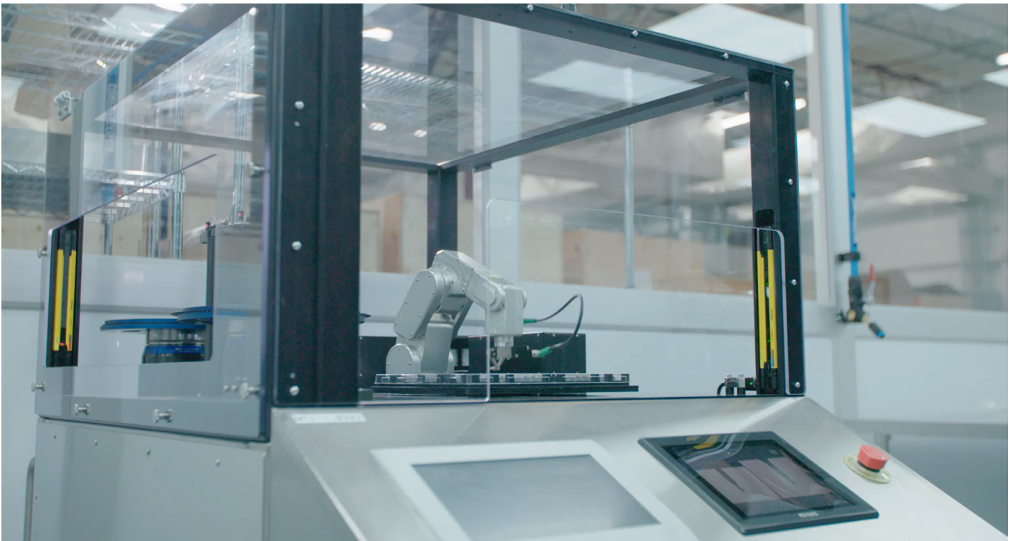
Figure 3: The Meca500 must be operated inside a safety enclosure (photo courtesy of Mati Therapeutics)
